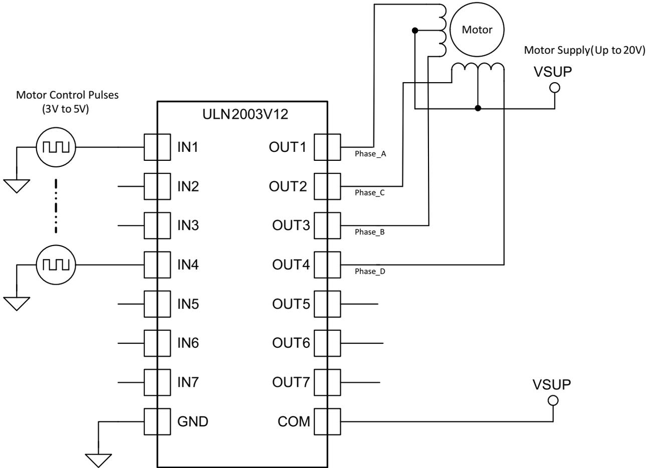
Figure 7. ULN2003V12 as a Stepper Motor Driver
