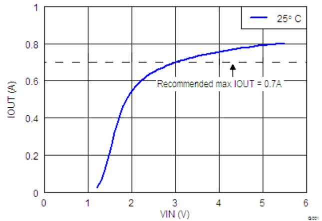
Figure 10. Load Current 7-Channels in parallel; VOL=0.6V
