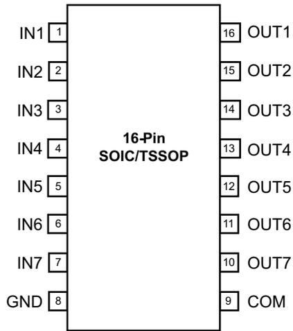
Figure 1. ULN2003V12 PINOUT
